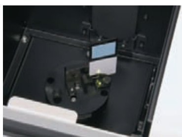
Irradiation of 980 nm laser light to up-conversion phosphor
